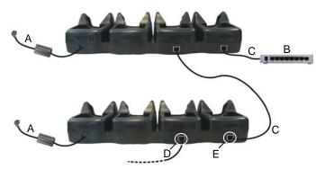
Figure 7 - Daisychaining Ethernet Connection
