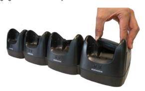
Figure 4 - Spare Battery Insertion
