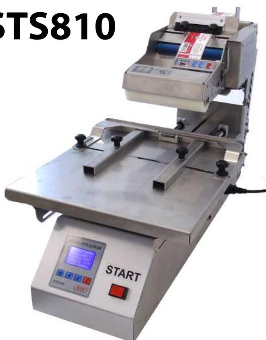
Semi-automatic labeling machine for gluing self-adhesive labels on a roll on flat-walled containers, rectangular, soft packaging and envelopes. Productivity of the machine from 450-700 pcs./hour depending on the length of the label and the speed of the operator. The containers are placed on the work platform and a robotic arm feeds and sticks the label on the container. All irregular form containers can be glued through matrix/mold.
