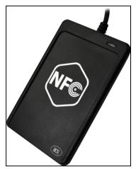
The ACR1251U is a PC-linked NFC smart card reader developed based on the 13.56 MHz contactless technology. Following the ACR122U, ACS's successful NFC reader and also the world's first CCID-compliant contactless reader, the ACR1251U offers more and advanced features. It is designed to support not only ISO 14443 Type A and B cards, but also MIFARE®, FeliCa and all four types of NFC tags and devices.
