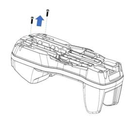
2. Unlock the lever and remove the connection module from the cradle.
