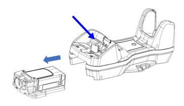
Replace the module by inserting it into the cradle, lock the lever and screw the module to the cradle.
