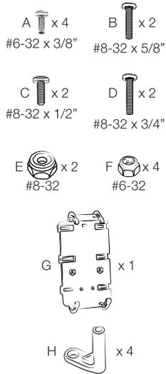
**1** Insert phone into main body (G). Determine best placement of fingers (H) to avoid blocking any buttons.
