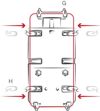
**2** Remove phone and attach fingers using small screws (A) and nuts (F).
