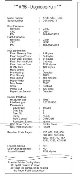
When the printer is configured for USB, this location will show either: "USB Driver Type: Native", "USB Driver Type: Printer Class", or "USB Driver: Comm Class".
