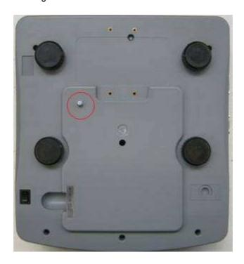
c) Level the platform by adjusting the adjustable feet until the bubble is in the centre of the level. The stability of the platform is very important.
