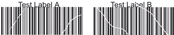
Possible printouts due to ribbon wrinkling
