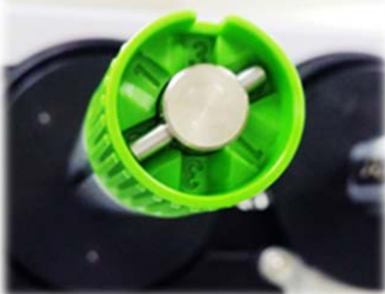
Ribbon Rewind Spindle Tension # 2
