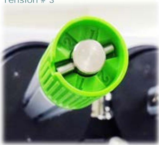
Ribbon Rewind Spindle Tension # 3
