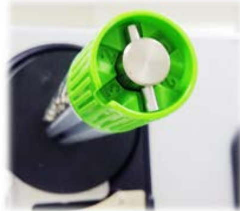
Ribbon Supply Spindle Tension # 1
