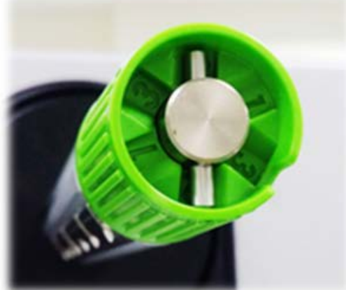
Ribbon Supply Spindle Tension # 2
