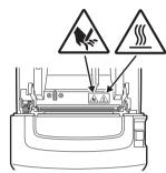
THIS LABEL INDICATES THE RISK OF BURNS DUE TO THE HIGH TEMPERATURE OF THE PRINT HEAD AND A RISK OF BEING CUT BY THE MANUAL AND AUTO CUTTERS WHILE THE PAPER COVER IS OPEN.
