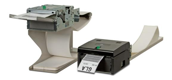
These ticket printers print on most ticket media from 50 mm to 82.5 mm wide using direct thermal printing. The ticket media can be up to 0.25 mm thick, fanfold, roll, or single cut handfed.
