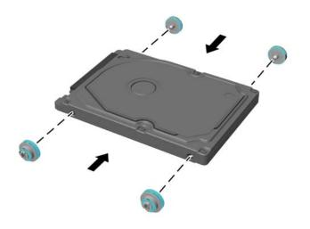
6. Align the guide screws with the slots on the chassis drive cage, press the HDD down into the cage, then slide it forward until it stops and locks in place (1).
