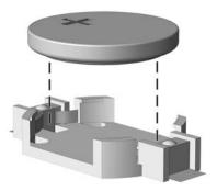
8. Slide the replacement battery into position, positive side up. The battery holder automatically secures the battery in the proper position.
