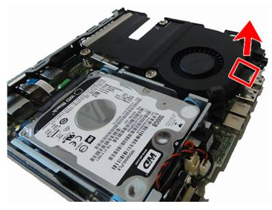
4. Disconnect the fan plug from the system board, and then lift the fan out of the chassis.
