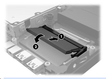
NOTE: A memory module can be installed in only one way. Match the notch on the module with the tab on the memory socket.
