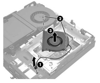
To install the secondary fan, reverse the removal procedure.
