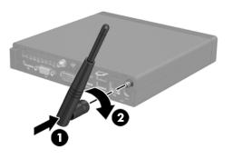
**11.** Connect the external antenna cables to the WLAN module.
