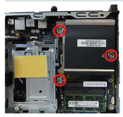
To replace the heat sink, reverse the removal procedures.
