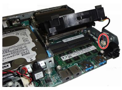
To install the fan, reverse the removal procedure.
