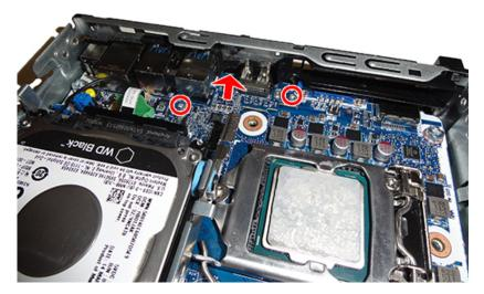
To install the expansion connector board, reverse the removal procedures.
