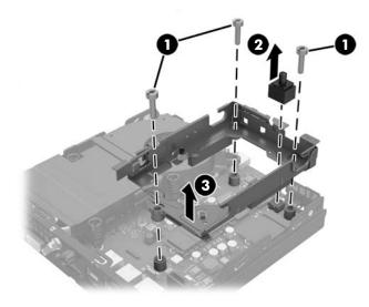
To install the drive cage, reverse the removal procedure.
