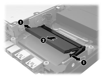
6. Slide the new SODIMM into the socket at approximately a 30° angle (1) then press the SODIMM down (2) so that the latches lock it in place.
