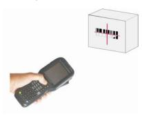
The Falcon X3 Imager uses an intelligent aiming system pattern, similar to those on cameras, indicating the field of view, which should be positioned over the code:
