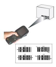
The XLR engine includes a pointer mode that projects a highly visible scan line at longer ranges to make it easier to accurately target bar codes. The user simply holds the trigger down until the aimer is on the appropriate code. Releasing the trigger then initiates the bar code scan.
