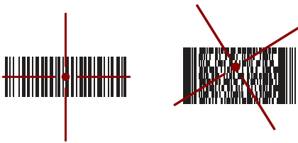
Figure 3-4 Imer Aiming Pattern: Bar Code Centered
