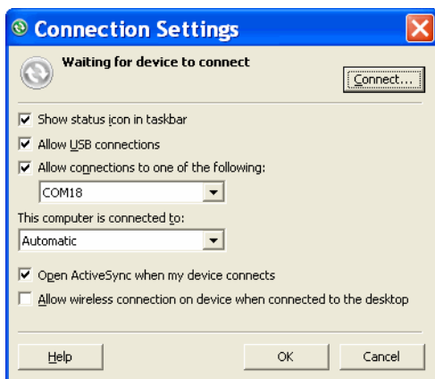
Figure 4-10 ActiveSync Connection Settings
