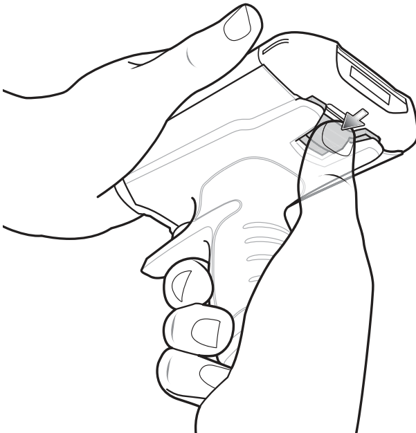
Figure 6-50 Press Release Latches
