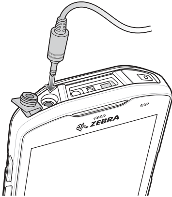
Figure 6-31 Audio Adapter Installation
