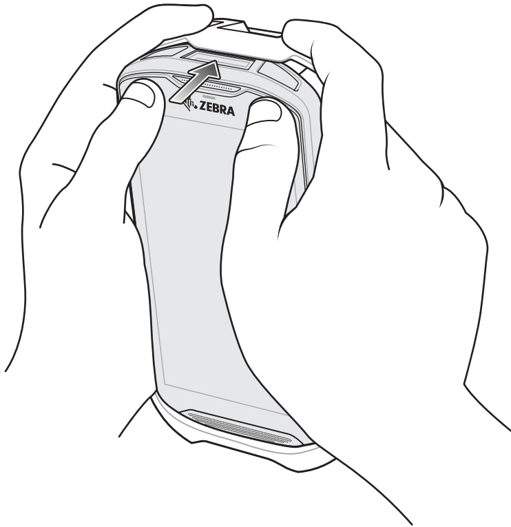
Figure 6-18 Push Device into Boot
