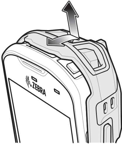
Figure 6-45 Lift Boot Over Device
