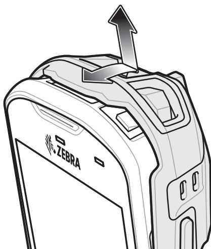
Figure 6-17 Lift Boot Over Device
