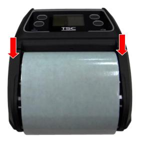
Press each side of media cover to close the media cover and make sure the media cover closed correctly.
