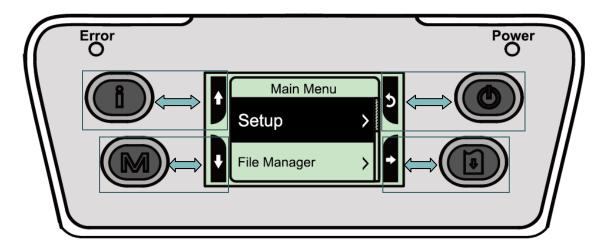
You can use this 4 buttons to scroll, select, enter or return the menu, depend on the icons from 4-sides of LCD. It was selected if the item with the black ground on the screen. The icon function is listed as below,
