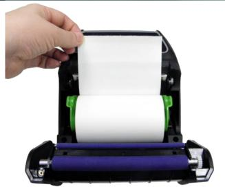
3. Place the paper, printing side face up, and pull out enough paper over the print head.
