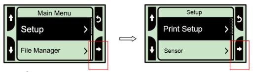
2. Press button to enter the "Print Setup" item. Select the "TSPL2" item. Enter the "Speed" setting mode.
