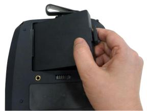
Insert the left side to install the battery at the rear of the printer.
