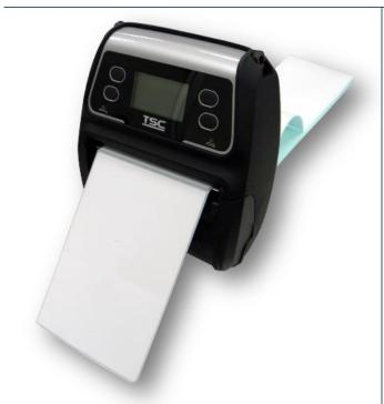
4. Press each side of media cover to close the media cover and make sure the media cover closed correctly.
