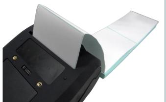
3. Feed the media through the rear external label entrance chute. Place the paper, printing side face up.
