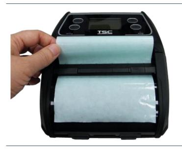
4. Feed the liner go through the peeler module. (as figure shown)
