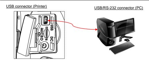
Open the interface cover and connect the printer to the computer/smart phone (host terminal) with USB cable. (USB to USB or USB to RS-232)
