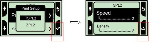
3. At this status, you can scroll up or scroll down to select the value of print speed. Then press the button to save the selected value into the printer. Press "butter to back to "Ready mode".
