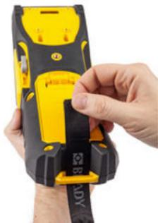
2. Still on the back of the printer, feed the strap under the loop at the top of the printer, directly into the media well.
