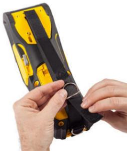
5. Weave the loose end of the strap back over the first (bottom) ring, then under and through the second (top) ring.
