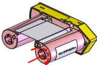
2. Carefully slide the ribbon cartridge into the printer until it seats firmly against the metal frame, then flip the printhead lock lever forward (to the left) to re-engage the printhead.
