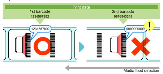
• A reading error occurs if the number of barcodes in the print data is not read within the printing period from start to finish and the timeout period (up to 2 seconds), even if the read results of the printed barcodes do not match the barcode data in the print data.
