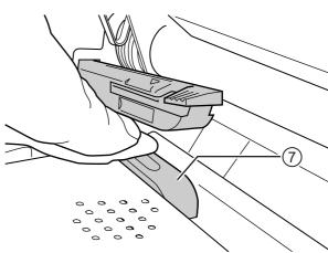
**9** Return the **media sensor guide** to its original position and tilt the **sensor guide lock** up to the locked position.
