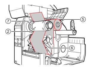
**6** Wind the ribbon counterclockwise to the **ribbon rewind spindle** ② and **grip sheet** ③.
