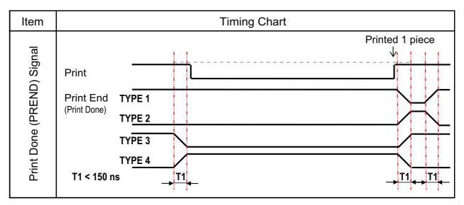
Rise or fall time (T1) of Print Done signal is less than 150 ns. You have to consider the time when outputting the signal from the connected devices.
