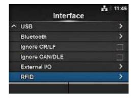
**7** Press the ▲/▼ buttons to select the item you want to set. Then press the ← button to go to the adjustment screen.
