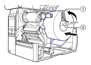
**6** Pass the media below the media damper (5) and media sensor guide (6) while pushing the media to inside of the printer. Make sure that the end of the media extends out the
