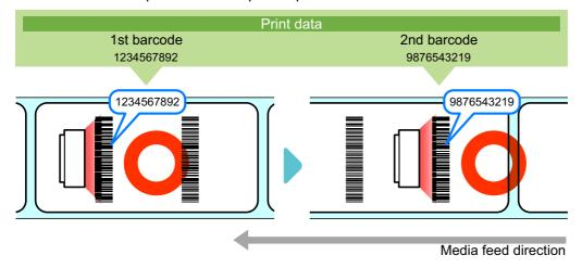
• A comparison error occurs if the read results of the printed barcodes do not match the barcode data in the print data.
