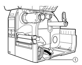
6 Press the **print head** down until you lock the **head lock lever** in place.
