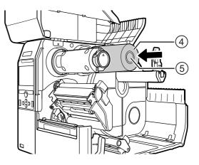
**5** From the **ribbon supply spindle** ⑤, pass the ribbon below the **print head** ⑥.
