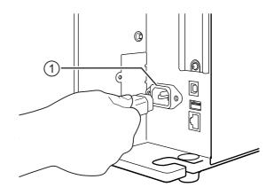
**2** Insert the power plug into an AC outlet.
