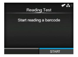
If reading is successful, the barcode type and data read are displayed on the screen. Only the first 23 bytes of data are displayed.
