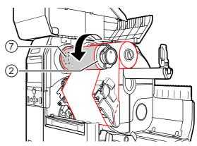
7 If the media is already loaded, press the print head down until the head lock lever is locked.
