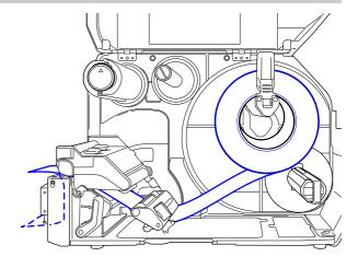
**2** Press the **tab** ① at the front of the printer to open the **dispenser unit** ②.
