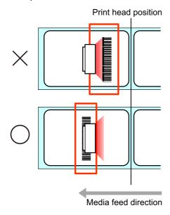
• Barcodes printed within the following range from the print end position cannot be read and a reading error inevitably occurs. As the following table is only for a reference, be sure to do a test read carefully in advance.
