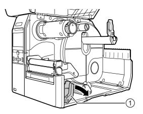
**5** Press the **lever** ② to remove the **print** head ③.
