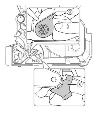
2 Clean the guide rollers ® using the cotton cloth dabbed with cleaning liquid.
