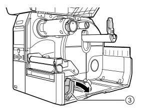
4 Load the ribbon @ onto the ribbon supply spindle ③.
