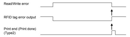
When the reprint count reaches the specified number, the RFID tag error and Machine error are outputted at a time. The machine error output is always a long pulse.
