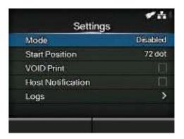
Fress the ▲/▼ buttons to select the mode for the barcode check function. The options are as follows:.
