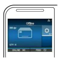
**2** Press the  $\circlearrowleft$  power button for more than two seconds to power off the printer.
