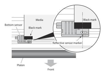
7. Lift the sensor arm up temporarily and adjust the media guide. Align the media with the fixed media guide on the left side, and then align the moveable media guide on the right side with the width of the media. Lower the sensor arm and fix the media in place.
