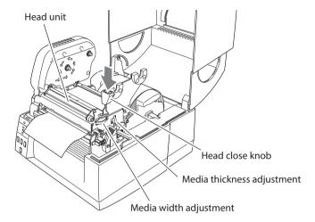
9. With the power switched on, push the FEED key to feed the media. It will halt at the next print start position.
