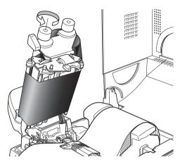
Ribbon Tension Adjustment (p.52) Ribbon Balance Adjustment (p.53) 7. Push the head close knob to lower and lock the head unit. Be sure to always push the head close knob to lock the head unit. If the ribbon is wrinkled, push the FEED key until the wrinkles disappear. If the wrinkles do not disappear or if it slips, perform ribbon balance adjustment and ribbon tension adjustment. See "Chapter 3 Printer Adjustments" for these adjustment methods.
