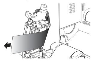
Using the adhesive leader of the ribbon or some adhesive tape, fix the ribbon that you have pulled out on the ribbon holder on which the paper core has been set and wind it on the ribbon holder.
