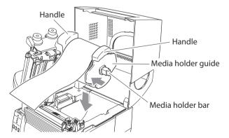
4. Set the media roll and media holder in to the printer as shown above. It is advisable to pull a length of media forwards and through the mechanism ready for later positioning. When lifting the media, use the handles on the media holder placed on either side.
