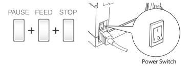
After the PRINT LED and CONDITION LED light up, release the keys to change the printer to sensor adjustment setting mode.
