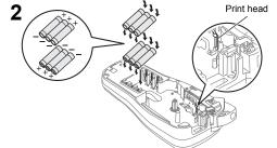
Insert six new AAA alkaline batteries (LR03) or fully charged Ni-MH batteries (HR03), making sure that their poles point in the correct directions. Users of alkaline batteries: Always replace all six batteries at the same time with brand new ones. Users of Ni-MH batteries:
