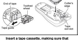
it snaps into place. · Make sure that the end of the tape feeds under
