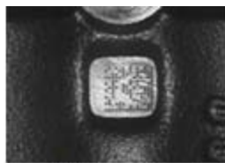
Dot Peening On Scratched Surface
