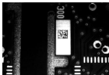
Figure 19 – Dot Matrix Code Directly Marked on PCB Copper Pad by Using Ink-Jet Technology
