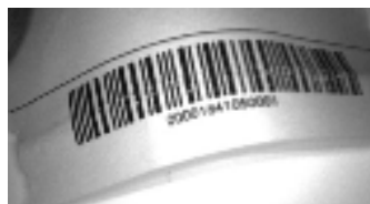
Figure 15 – Barcode Printed on Curved Surface Readable by Matrix 300N in spite of Image Optical Distortion
