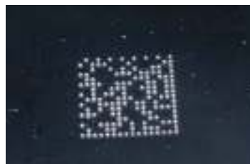
Figure 18 – Directly Marked Dot Matrix Code Characterized by Outstanding Separation Distance between Adjacent Code Elements
