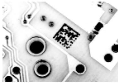
Figure 20 – Data Matrix Code Directly Marked on PCB Surface by Using Laser Etching Technology
