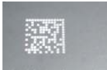
Figure 17 – Dot Peening Marking on Metal Surface with Multi-dot per Code Element
