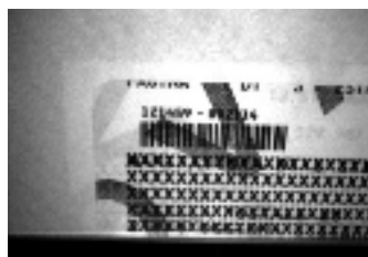
Figure 14 – Overprinted Barcode Readable by Matrix 220 also Through the Envelope Window Film
