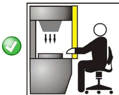
Figure 2 - Correct light curtain positioning
