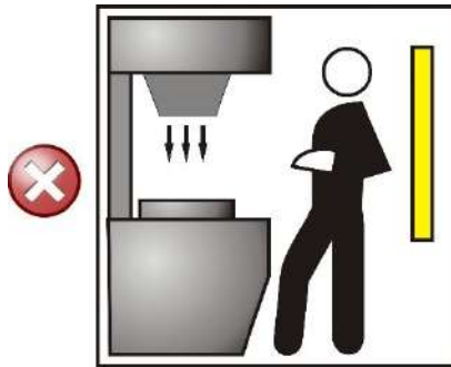
Figure 3 - Wrong light curtain positioning
