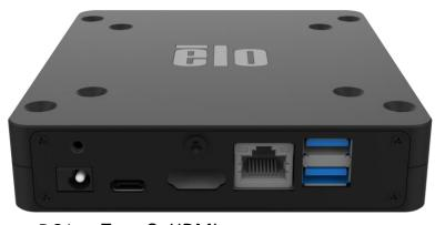
DC In Type C HDMI Ethernet USB 3.0
