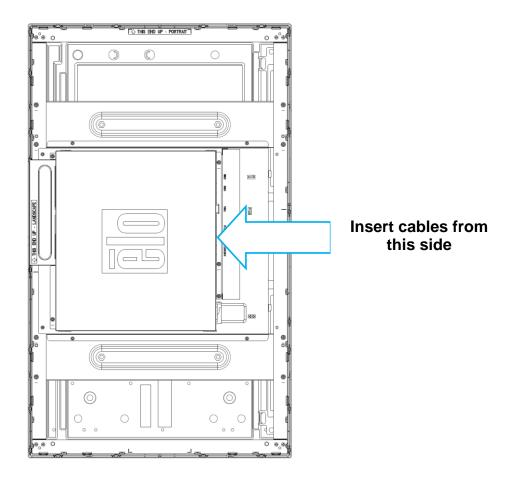
Landscape mode can only be installed at 0 degrees such that the Elo logo is on the back is not rotated and the cables are connected from the bottom, as the image below shows.
