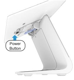
Power on the system when installation is complete.
