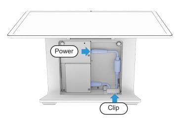
Route the DC power cable through the hole in the bottom of the stand and connect it as shown. Connect other I/O cables as needed (see back page) Make sure all cables route through the plastic clip at the bottom. 3 Mount the system to a table (optional). Skip to Step 6 if not mounting to a table.
