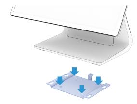
Secure the mounting bracket to the table using appropriate screw type and length. Elo suggests M4 or #10 screw diameter.
