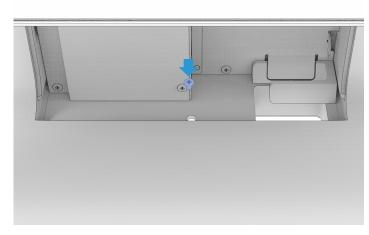
Secure the system to the bracket using the screw included in the accessory box.
