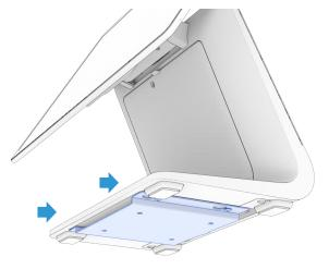
Lower the system onto the bracket and sldie it back ensuring the bracket engages the screws on the bottom side. ļ
