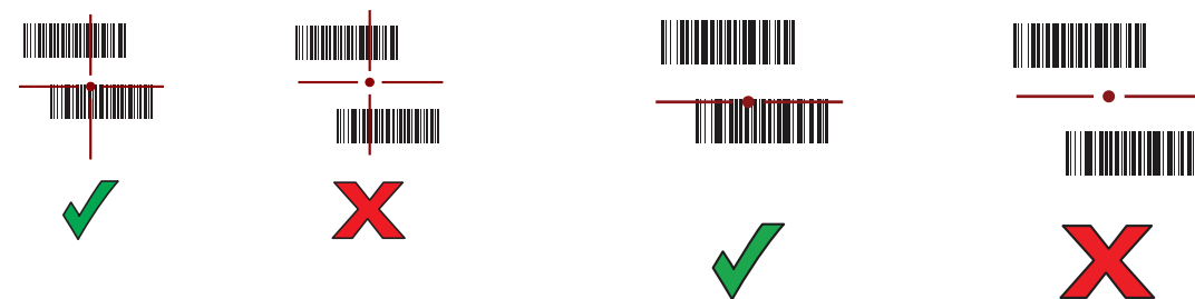
Figure 74 Pick List Mode with Multiple Barcodes in Aiming Pattern: Standard and Extended Range
