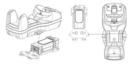
7. Move the base station up until the sphere is aligned with the smaller hole, then lock the lever to secure the connection module.
