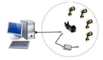
In stand alone systems, each base station is connected to a single Host.
