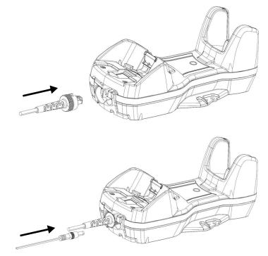
After connecting the power supply cable, secure it on the strain relief as shown in the figure below.
