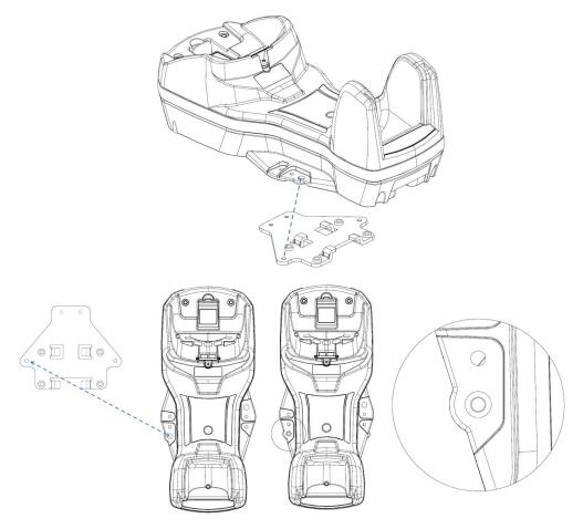
4. Move the base station down until the sphere is aligned with the smaller hole.
