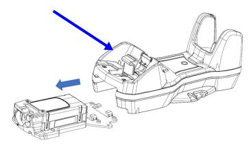
5. Screw the connection module and mounting plate sub-assembly to a flat surface using four screws as shown in the figure below.
