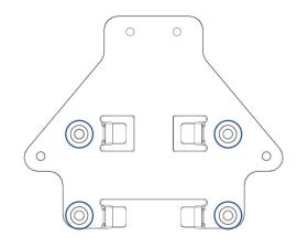
2. Remove the adhesive strips protecting the mounting tabs on the base station.
