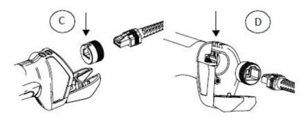
4. Once the cable is properly inserted, close the handle and screw it back into the body.
