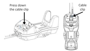
3. Pull out the multi-interface cable and put the lever back into lock position.
