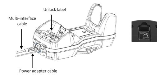
The BC9631 (BC9600 + CM9631 connection module) provides a single multi-interface connector. Power is supplied by the host (USB) or by an external power supply connected to the cable.
