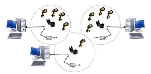
Many stand alone connections can operate in the same physical area without interference, provided all readers and base stations in the system have different addresses.
