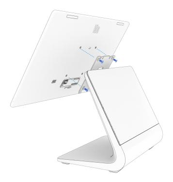
4 Mount the system to a table (optional). Skip to Step 6 if not mounting to a table.
