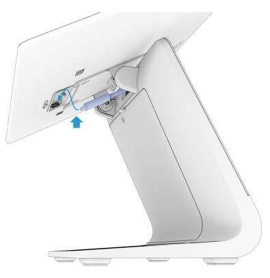
8 Slide the upper VESA mount cover over the VESA mount bracket and install the M3x6mm screw removed in step 2 to secure it in place. Install the lower VESA cover so it covers the USB-C cable ensuring the cable routes freely. Install the M3x13mm screws removed in step 2 to secure the lower VESA mount cover.
