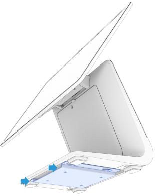
6 Secure the system to the bracket using the M4x8mm screw included in the accessory box.
