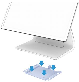
5 Lower the system onto the bracket and slide it back ensuring the bracket engages the screws on the bottom side.
