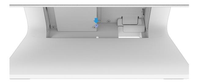
7 Connect the USB-C cable located in the hinge of the stand to the I-Series 4 Slate display. Re-install the cable lock bracket and screw from step 1.
