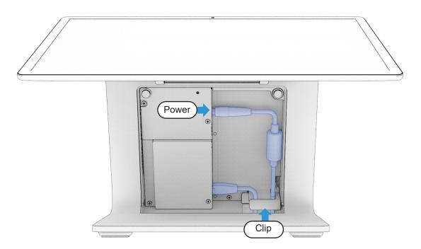
11 Power on the system when installation is complete.
