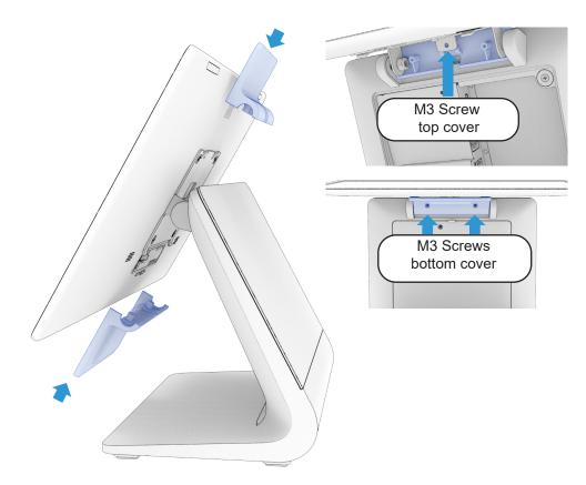
9 Remove the cable cover door to access the I/O connections.
