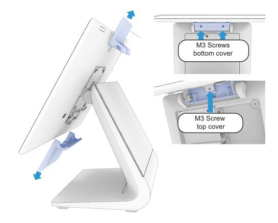
3 Install I-Series 4 Slate display on stand using included M4x6mm flat-head screws.
