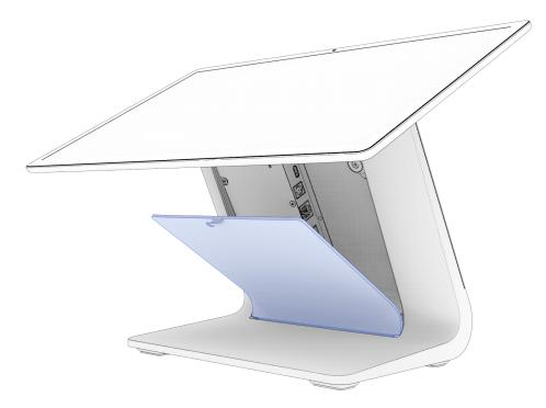
10 Route the DC power cable through the hole in the bottom of the stand and connect it as shown. Connect other I/O cables as needed (see page 2) Make sure all cables route through the plastic clip at the bottom and re-install cable cover door.
