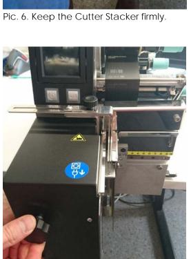
Pic. 8. Support the Cutter Stacker with one hand and tighten the screw with your free hand.
