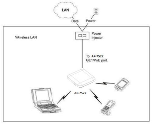
The Power Injector can be installed free standing, on an even horizontal surface or wall mounted using the power injector's wall mounting key holes. The following guidelines should be adhered to before cabling the Power Injector to an Ethernet source and an Access Point:
